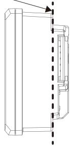
太線(青)の内側: 埋め込み部分の外形ライン The inner side of the heavy line (blue): outline of the embedded part
