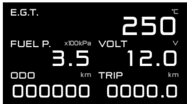
If the sensor of the displayed item is not connected, "x" is displayed in the zone.
