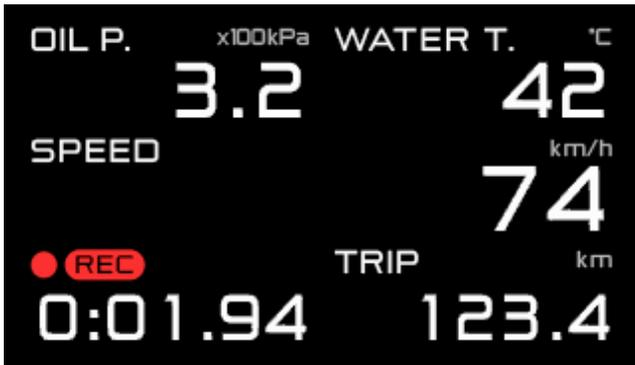
This mode records the driving data for up to 3 minutes. During the record mode, [●REC] is displayed in the multi-display zone.
