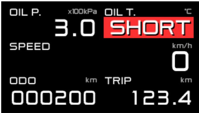
If the sensor is open or short circuit, the corresponding display item will turn red background and show [OPEN] or [SHORT]. Once [OPEN] or [SHORT] is displayed, it will remain displayed until the ignition is turned off. Regarding the oil pressure and fuel pressure, [SHORT] is only displayed during a short circuit.
