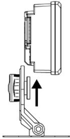
7. Adjust the angle and location to attach. The mounting bracket is bendable to fit on the place to attach.
