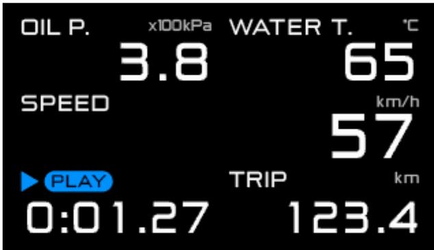
This mode plays back recorded data. Pause, frame advance, fast forward, frame back, and rewind are also possible. During the playback mode, [▶PLAY] and the playback time are displayed in the multi-display zone.
