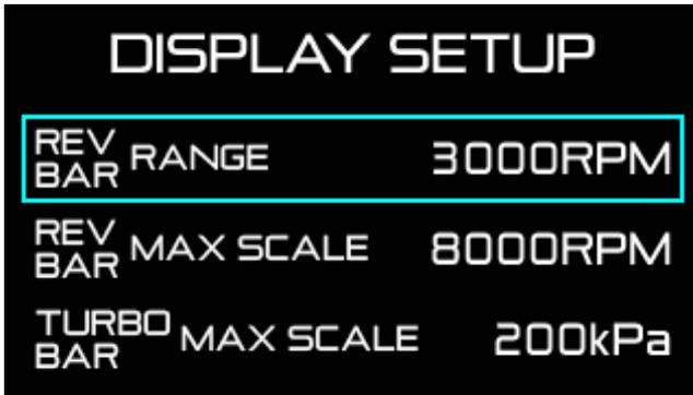
2. Press the **【F2 button】** to move the selection frame to the item you want to set, and press the **【F1 button】** to change the setting.
