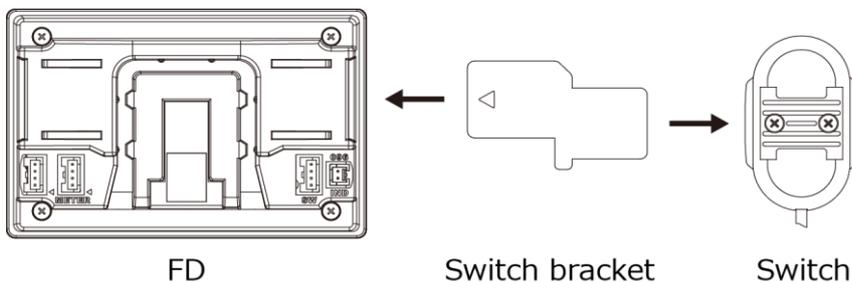
⚠ The side with the triangular (▷) hole comes to the FD body side.
