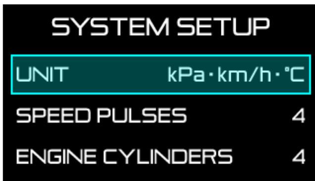
3. Press the [MIDDLE button] or [RIGHT button] to move to the setting item, and press the [LEFT button] at the item you want to set. The light blue color inside the selection frame will disappear and the setting can be changed.
