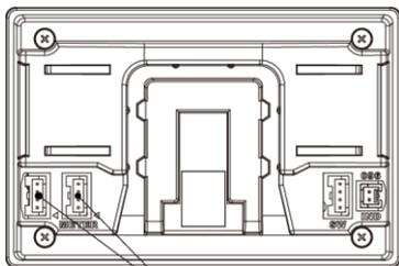
Connectors for meter wires (white)
