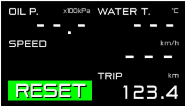
This mode resets the maximum value (maximum and minimum values for oil pressure and fuel pressure) of during driving and idling up to that point. During the peak reset mode, [RESET] is displayed in the multi-display zone for 1 second.
