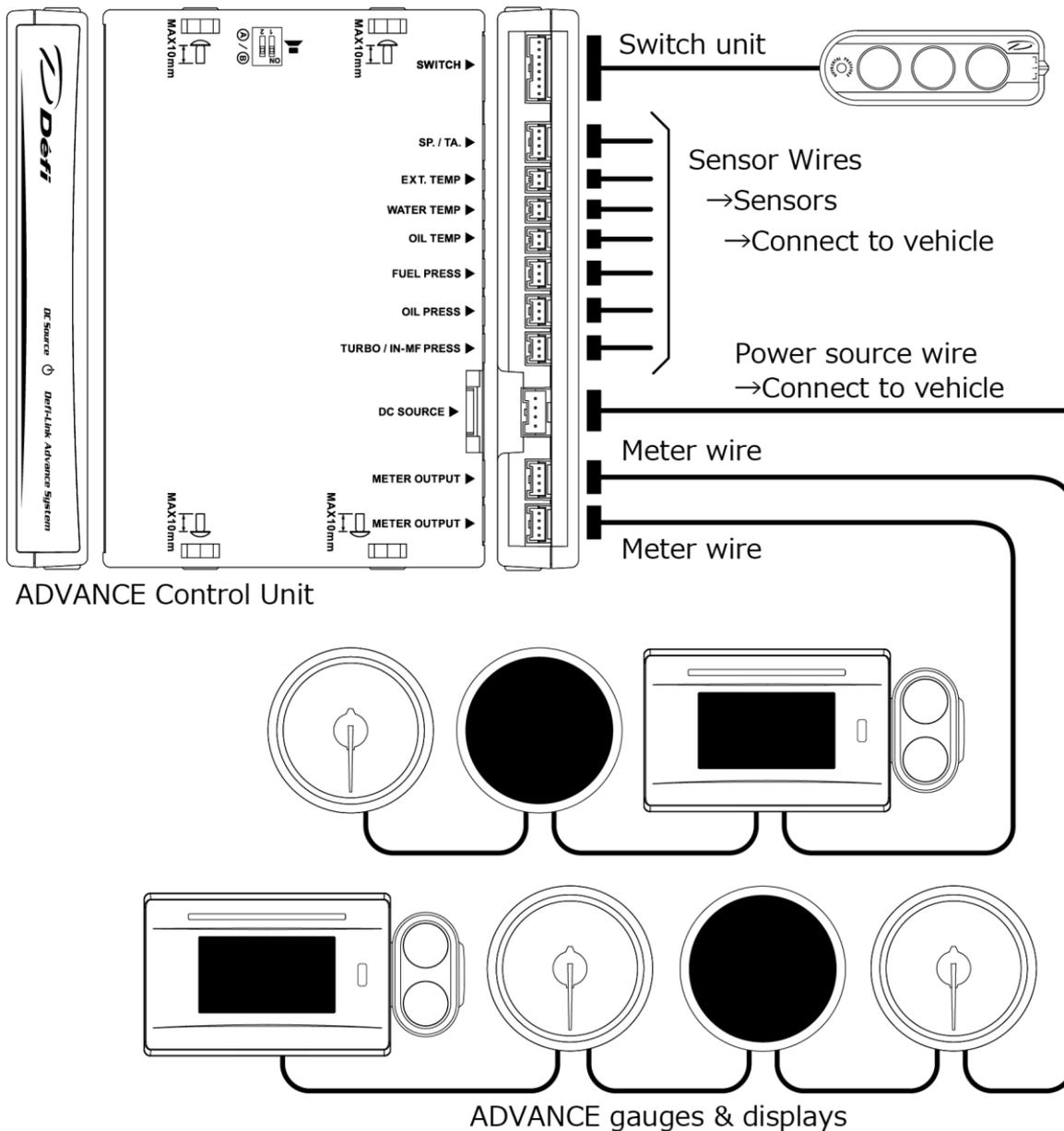
The meter wire can be connected to either of the two connectors of METER OUTPUT.
