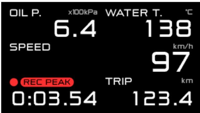
This mode displays the maximum values from the time that recording was started during the record mode. For oil pressure and fuel pressure, the maximum and minimum values are displayed in sequence. Even when differential pressure is displayed, the peak fuel pressure value is displayed in the fuel pressure zone. During the record peak mode, [●REC PEAK] is displayed in the multi-display zone.
