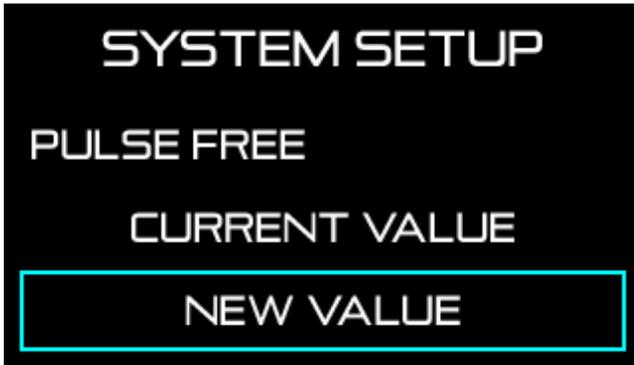
3. After [NEW VALUE] is selected, press [LEFT button] while the vehicle speed of the genuine gauge is 60km/h or 40MPH to complete the speed pulse setting.
