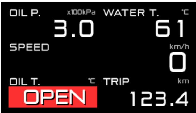
If communication between the FD and the unit is lost, [SERIAL LINE ERROR!] will be displayed.
