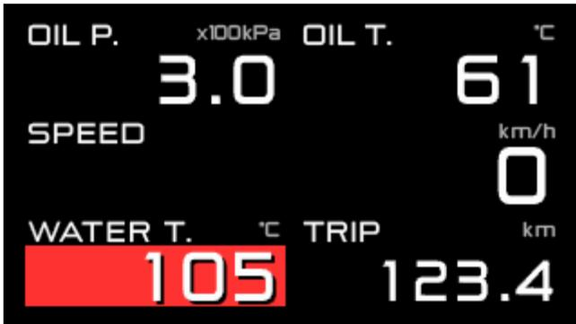
While the value exceeds the set warning value, the corresponding item in the digital display turns to a red background.
