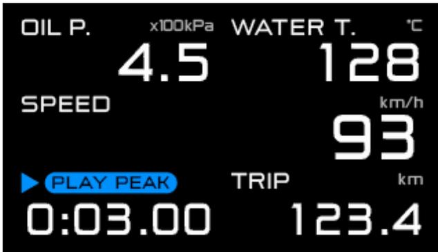
This mode displays the maximum values in the recorded data during the playback mode. For oil pressure and fuel pressure, the maximum and minimum values are displayed in sequence. During the playback peak mode, [▶PLAY PEAK] is displayed in the multi-display zone.
