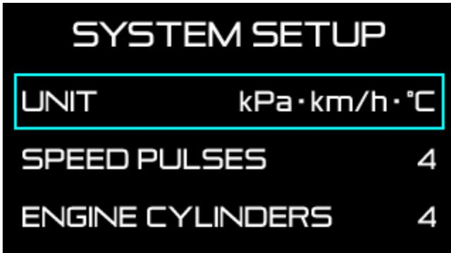
4. Change the setting with [MIDDLE button] or [RIGHT button], and press [LEFT button] to confirm the change. The inside of the selection frame turns light blue.
