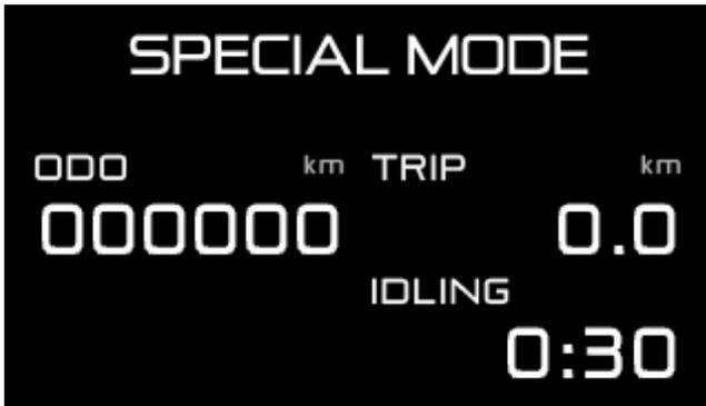
If the special display is set to [ON] in the system setup mode and the vehicle speed of 0 km/h (0 MPH) continues for more than 10 seconds, the special mode will be shown. During the special mode, the odometer, trip meter, and idling time are displayed.
