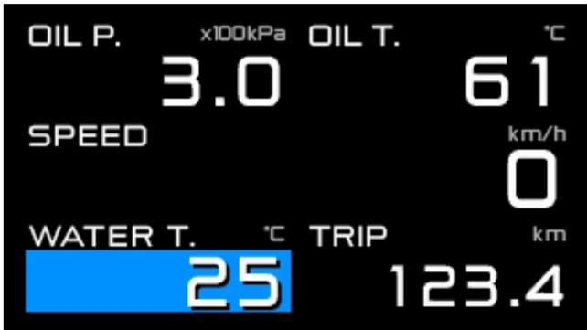
If the warm-up mode is set to water temperature or oil temperature in the system setup and the actual temperature is lower than the set temperature, warm-up is displayed.
