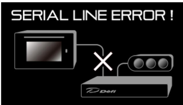
If an error is displayed, turn off the ignition immediately and check the sensor and wiring. If any defects are not found, ask the shop where the products were installed for inspection.
