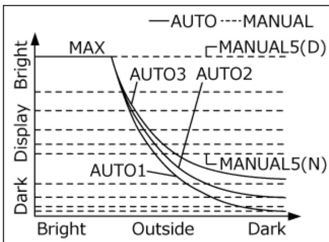
The illumination of all the connected gauges is controlled automatically by connecting FD and ADVANCE gauges in one ADVANCE System and by using the [AUTO] as follows:
