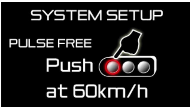
4. If the speed pulse is within the setting range, a buzzer sounds and [COMPLETED] is displayed. Press the [LEFT button] to confirm. If the speed pulse is out of the set range, [INCOMPLETED] will be displayed. Press the [LEFT button] to return to the setup screen.
