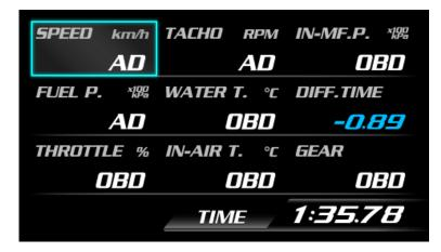
When digital gauges are displayed on the screen, the signal sources ("AD" or "OBD") are shown by touching the screen or pressing the ENTER/MENU switch.
