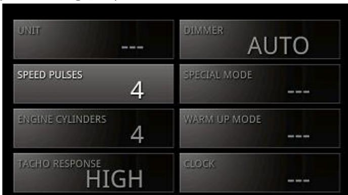
Selecting an item by using “UP” or “DOWN” switch on the ADVANCE Control Unit Switch and pressing WARN SET, you can change setting items.
