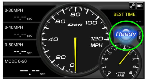
After you stop your vehicle completely, please touch “Measurement”, and then “Ready” message will appear. The time measurement will start automatically when your vehicle is in motion. Once you reach your set speed, the measurement will be stopped automatically.
