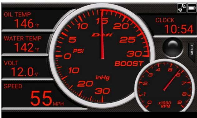
『HUD Display』 : Ticking the checkbox, gauge illustration on the screen will turn to the inverted mirror image for Head Up Display. During nights, you can reflect it on your windshield.
