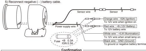
**•** When several gauges are installed into a vehicle, use each power supply wire to connect gauges to the vehicle independently. Do not join multiple power supply wires. Do not share single fuse with multiple gauges. Every gauge requires independent fuse for IGN and +B line.
