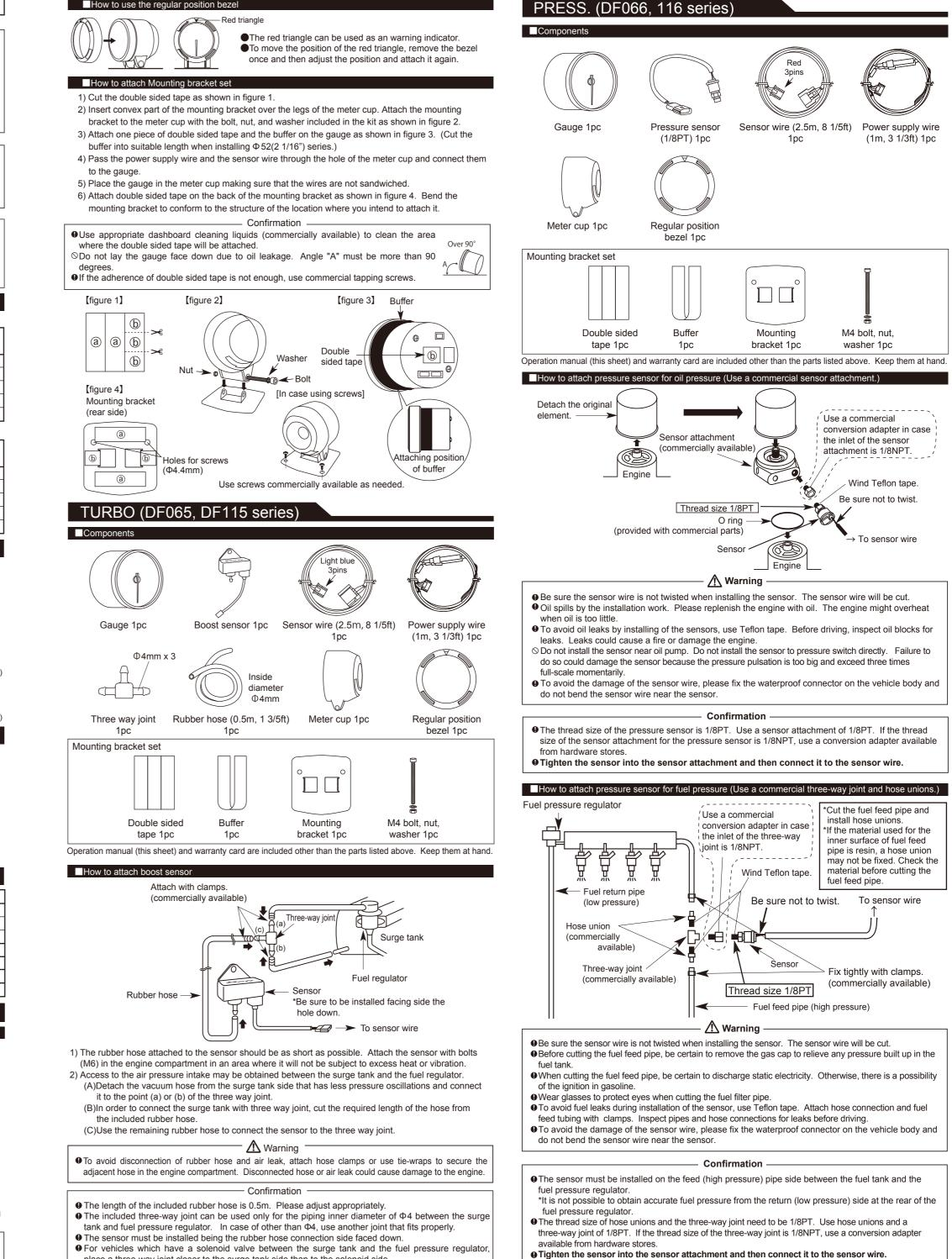
place a three-way joint closer to the surge tank side than to the solenoid side.
